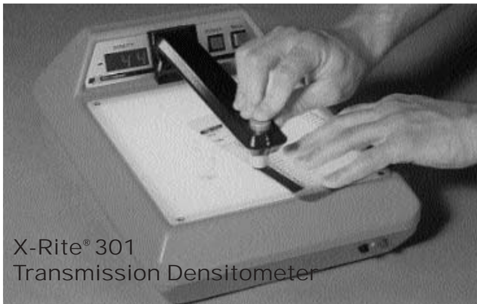
The Model 301 has an easy-to-read display, lighted work surface, and simple calibration.
